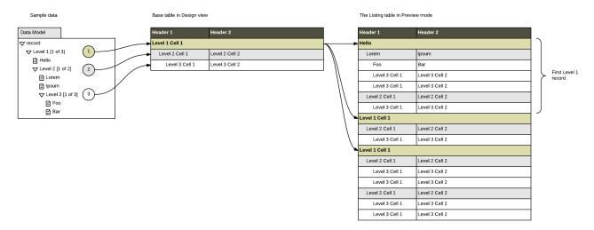
At this stage there is no user interface to configure this type of dynamic table but in a separate Technical article. It can be achieved by setting some HTML attributes in the *Source* view and adding scripting to populate the cells.
